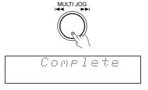
When the recording level adjustment is completed, stop playing the source.
